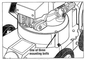
Figure 32: Engine mounting bolts.
